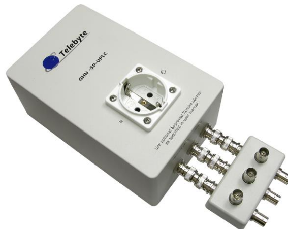
The GHN-SP-UPLC connected to the GHN-SP-SPLCOMB-UPLC-3
